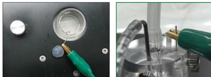
Reducing a stimulation artifact by a platinum wire. Examples without (left panel) and with (right panel) a MED perfusion cap
