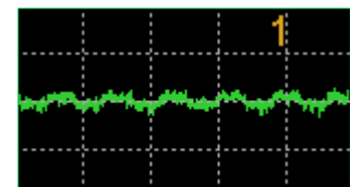
An example of magnetic field noise caused by an incubator. Interference occurs in particular electrodes, the magnitude of effect depends on the position in the incubator, and the noise disappears when the temperature is stabilized (an example screen of the MED64-Basic to clearly show the disproportionate effect).
